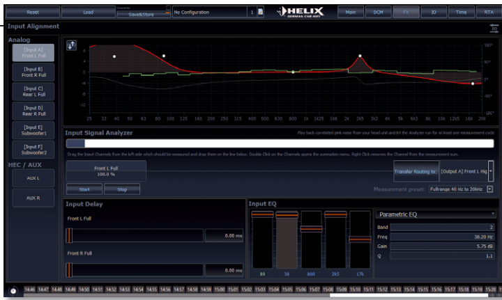
The inputs can be measured in the ISA (Input Stage Analyzer) and corrected directly using the runtime and equalizer
