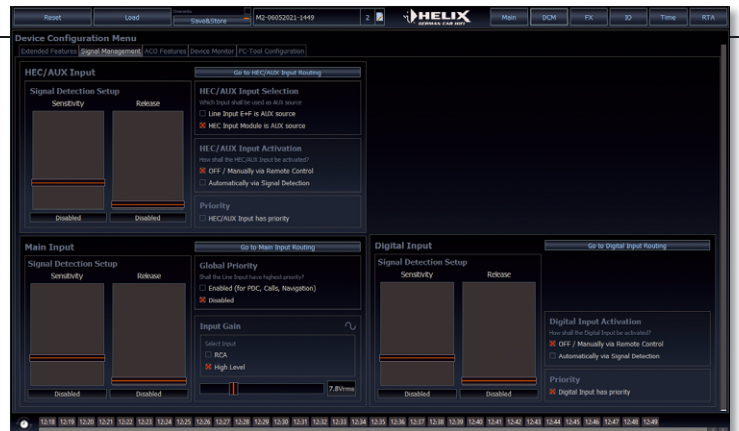
The prioritization options for the individual sources are exemplary. Now there is also a channel-pair sensitivity adjustment with clipping display
